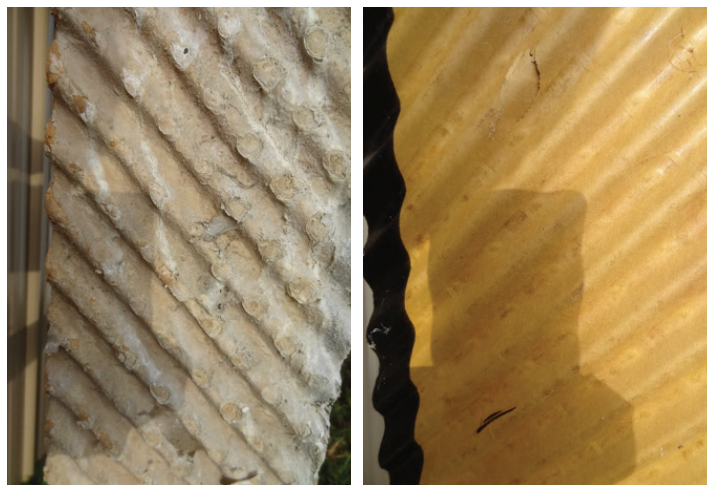
Figure 5. While the front of the pad may look clean, the flutes within the pad can be much dirtier resulting in air restriction that people may not be aware is there.
